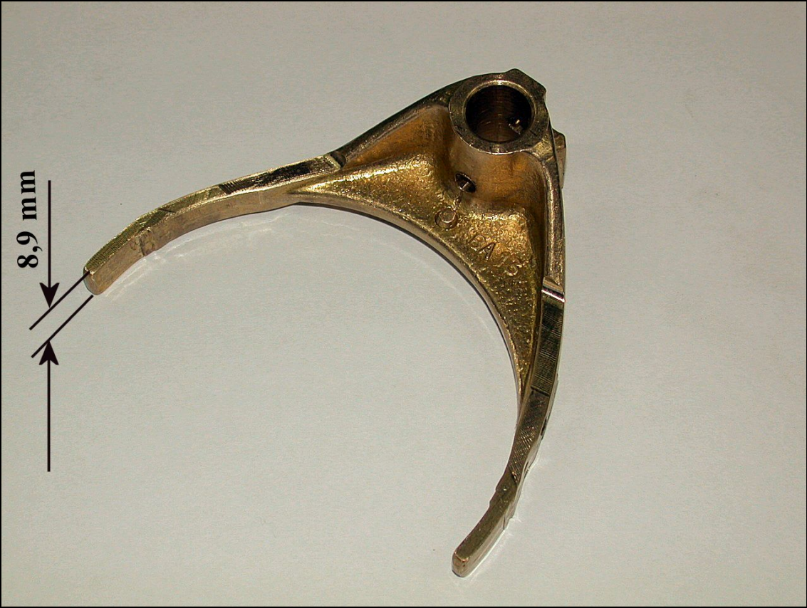
Photo n°2 – The 1 st – 2 nd gearshift fork after the face milling required.
